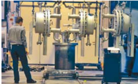
480 kW Raffinate Stripper Bottoms Cooler, PSHE 5HH-148/1/1
