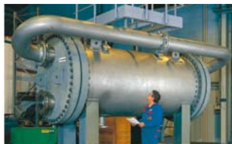
30 MW Effluent Economiser at Ethylene Oxide Plant, PSHE 14HH-968/2/2
