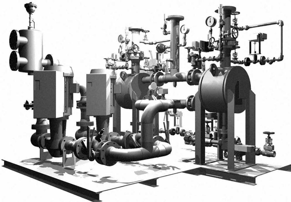
Vahterus provides Plate & Shell Heat Exchanger design for building-heat packages manufactured by Preston Phipps. The compact design makes it possible to manufacture skid assemblies that can handle large loads and take up a much smaller footprint.
